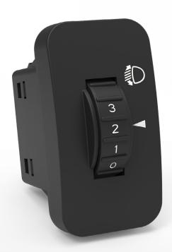
The CVR-Series is a configurable three- or four-position rheostat switch designed for vehicle lighting control. Available for 12VDC and 24VDC systems, the CVR-Series automotive rheostat switch is made with durable thermoplastic materials and silver-plated brass terminals for reliable operation in commercial vehicles, such as work trucks, agricultural equipment, and construction equipment. The front panel-mount dimmer switch is available with or without white backlighting.
